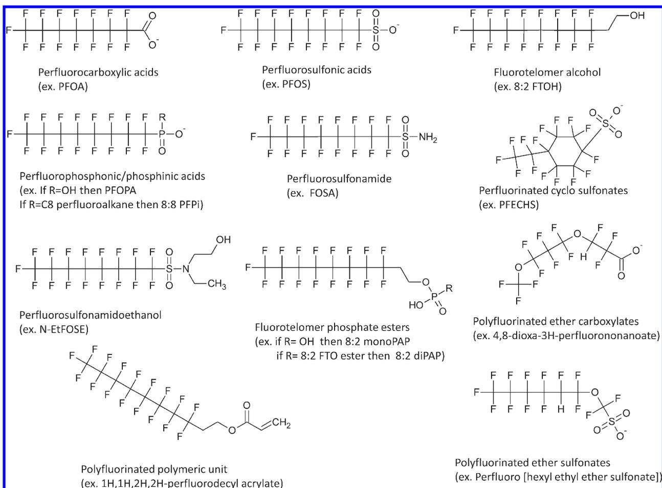
**Figure 1.** Generic structures for polyfluorinated compounds. The  $n = 8$  linear carbon structures are shown for many of these examples, but  $n = 4-14$  linear and/or branched carbon units are generally possible.
